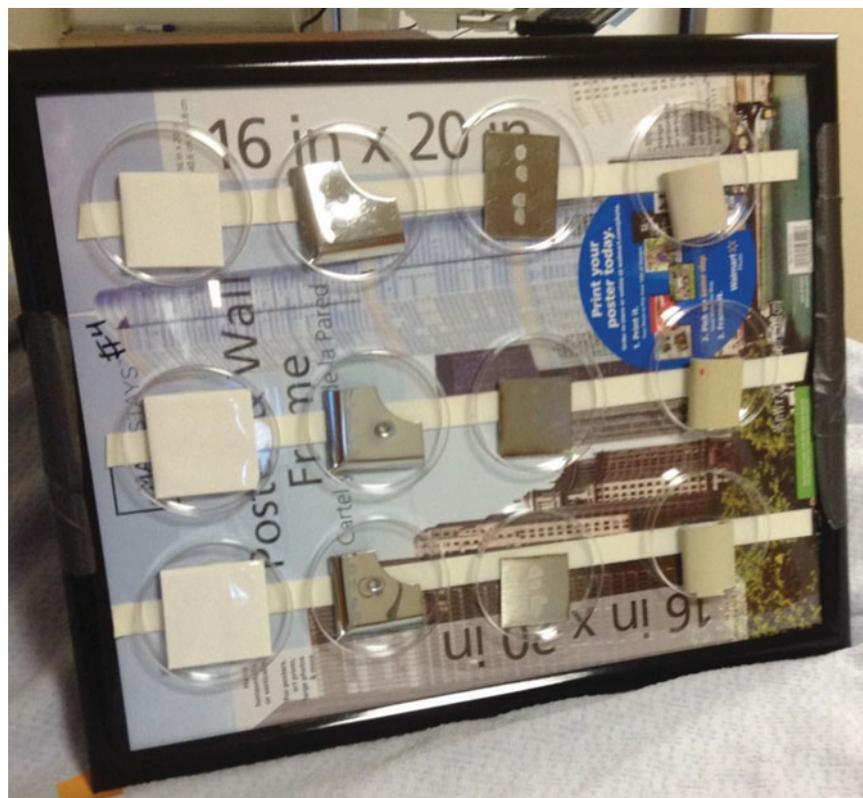
**Figure 2.** Surface coupons contained within petri dishes in triplicate placed onto vertical panel at site 3 on top of the patient bed within hospital room prior to UVGI treatment. Surface coupons from left to right: porcelain tile, chrome light switch cover, stainless steel, bedrail.
