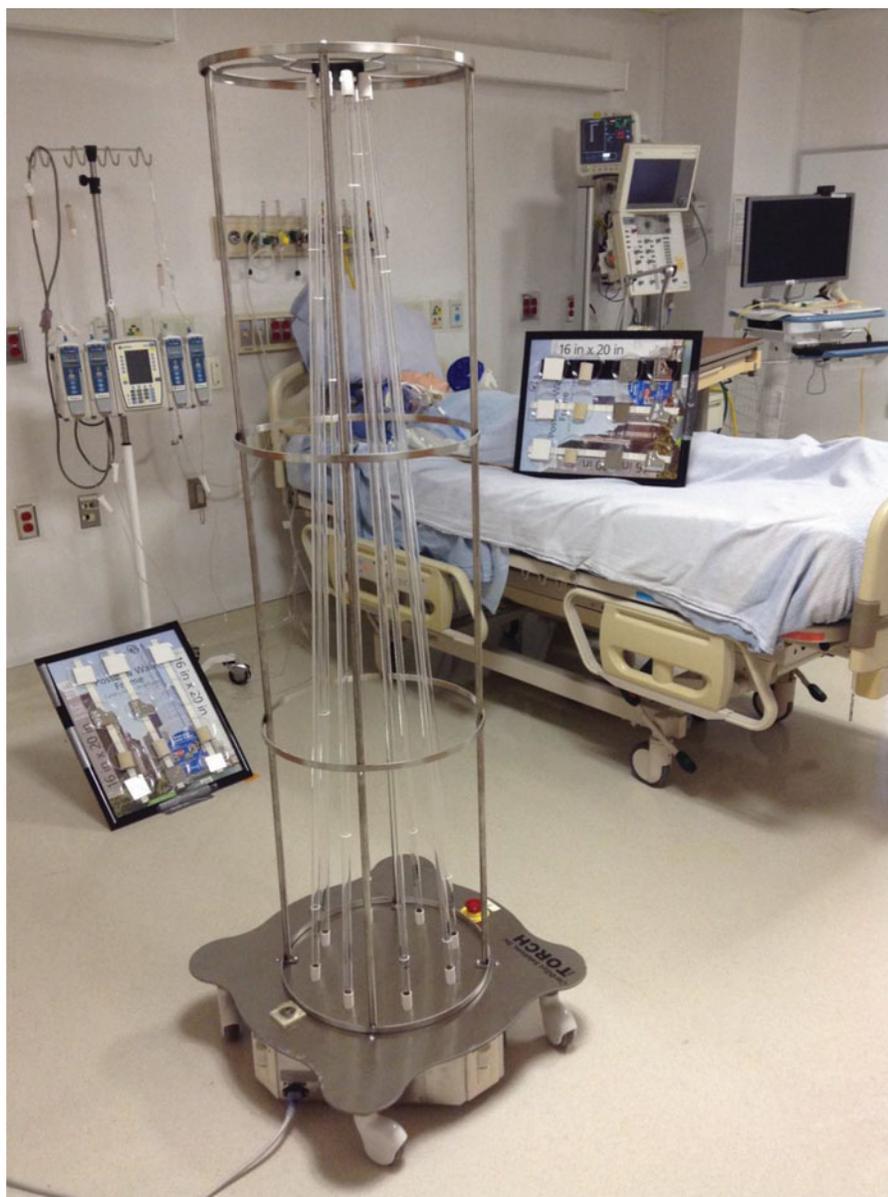
**Figure 3.** Ultraviolet germicidal irradiation (UVGI) portable generator and surface coupon/panel setup within hospital room for UVGI treatment. Surface coupons of each type are attached to panels at site 2 (floor next to UVGI generator) and 3 (top of patient bed) and placed vertically ( $\sim 60^\circ$ ). A mannequin was present on the patient bed during UVC exposures; however, personnel should be evacuated from the hospital room before UVGI use.
